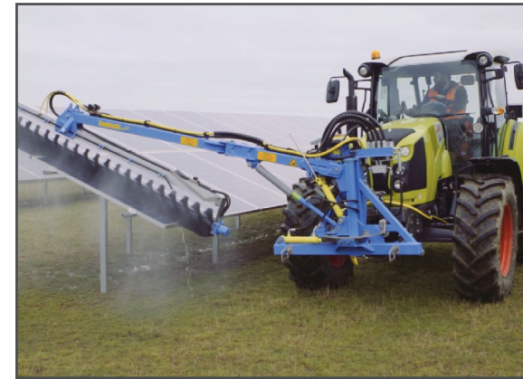
Plate 7.2 - Typical Solar Farm Cleaning Unit
